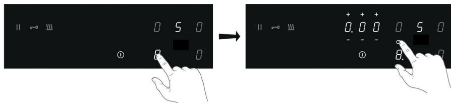
3. Use the '+' or '-' key to set the desired time (from 1 minute to 9 hours and 59 minutes).
