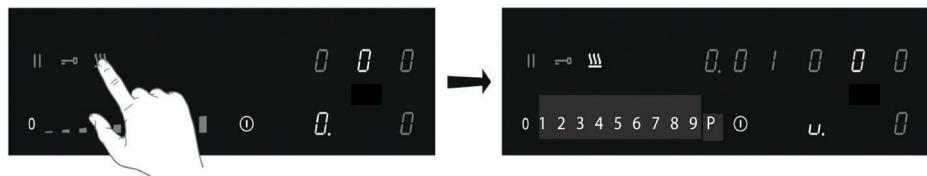
4. Set the power level to '0' or touch the keep warm key to switch off the keep warm function.
