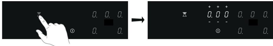
2. Use the '+' or '-' key to set the desired time (from 1 minute to 9 hours and 59 minutes).
